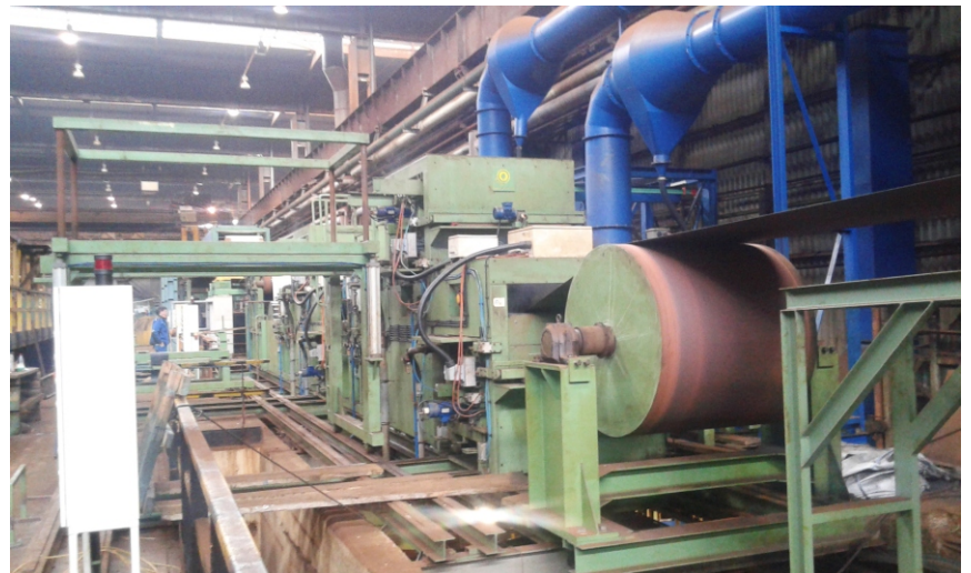
Photo above: 3D picture show a 15m high machine for coil steel strips mechanical cleaning. Slika zgoraj: 3D modelna risba prikazuje 15m visoko postrojenje za mehansko čiščenje trakov.
