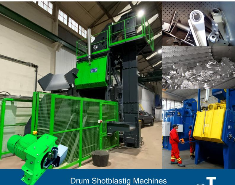
Machines are used for cleaning different work pieces of approximately the same size. Drum shot blasting machines can be also continuous. Machines are equipped with a rubber or a steel belt and are ideal for:
