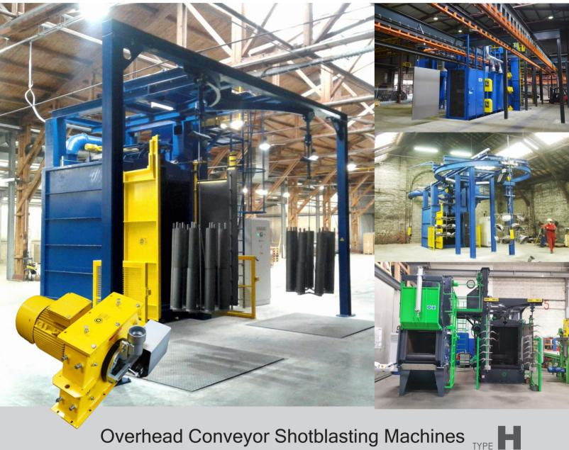
Parts can be hanged individually or in a tree on revolving hooks. Spinner hanger machine is ideal for:
